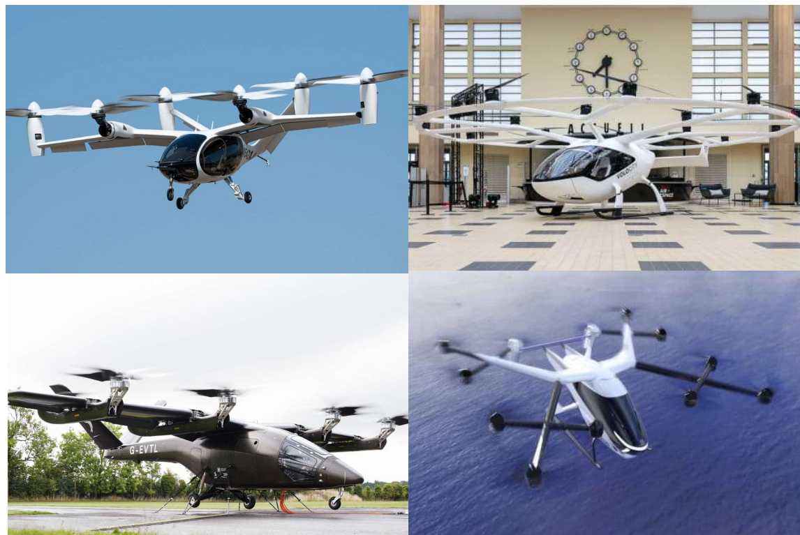
左上 : Joby Aviation "Joby S-4", 右上 : Volocopter "VoloCity" 左下 : Vertical Aerospace "VX4", 右下 : SkyDrive "SD-05" ( https://evtol.news )
